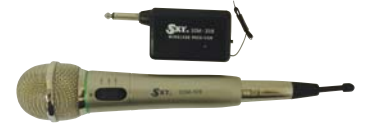
SDM-309 – HAND HELD WIRED OR WIRELESS MICROPHONE FREQUENCY RANGE: VHF/FM, FREQUENCY RESPONSE: 100HZ-10000HZ, S/N RATIO: 60DB, DIRECTIVITY: UNI-DIRECTIONAL, SERVICE AREA: 15 TO 30M, WIRED SENSITIVITY: -54DB+3DB, RECEPTION SENSITIVITY:30DB/UV
