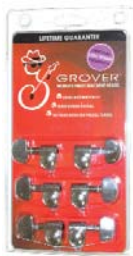
GROVER GUITAR LOCKING ROTOMATICS TUNING GEARS 18 TO 1 GEAR RATIO, SIMPLY INSERT STRING, PULL TENSION BY HAND AND BEGIN TUNING. AS YOU START TO TUNE, ONLY THE LOCKING CAM IN THE STRING POST TURNS. ONCE THE STRING IS LOCKED, THE STRING POST BEGINS TO TURN ALLOWING YOU TO BRING THE STRING TO PITCH. IN LESS THAN ONE REVOLUTION OF THE STRING POST, YOU WILL BE IN TUNE, TO STAY IN TUNE. LIFETIME GUARANTEE. WE HERE AT VJ'S NOW HAVE ACCESS TO GROVER PRODUCTS AND CAN RESTOCK QUICKLY AT LOCAL GROVER WAREHOUSE.
